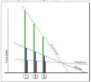
help me in explaining the relation between perspective and angle of view. So, if we consider that the objects 1, 2 and 3 on the diagram have similar height and the small green dot to be the point where all objects are seen as a dot, then there is a definite line along which the object change their sizes. And the line creates an angle, which I will call the perspective angle.
