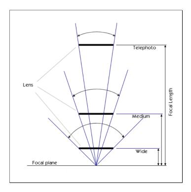
On the diagram above you may see the correlation between the focal length (the distance from the focal plane/point of focus to the lens). Usually there more then one piece of glass in the lens, but there is one plane that is considered to be the lens plane. So the angle is wider when the lens is closer to the focal plane (remember the name "wide-angle lens"?) and the angle is small when the lens are farther away.
